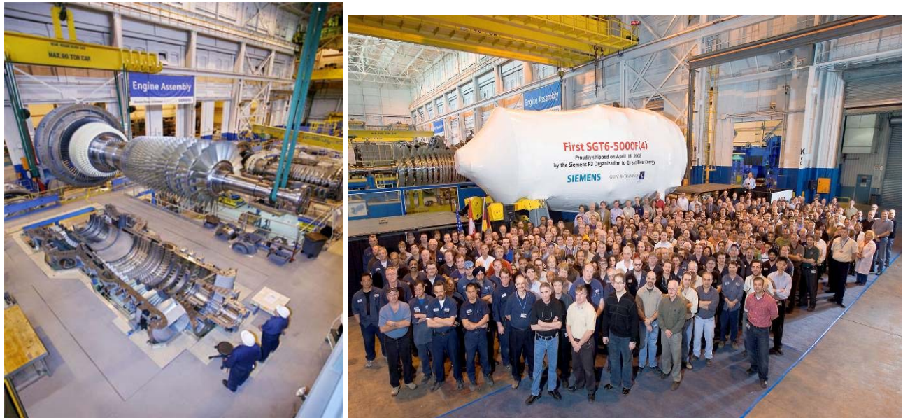
Siemens SGT6-5000F4 Gas Turbine Rotor, and Shipment from Hamilton
